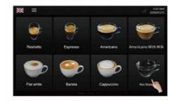
Step 2: During the beverage making process ... click on the "+" on the page to pop up the parameter adjustment pop-up window, click "-" or "+" to temporarily adjust the amount.
